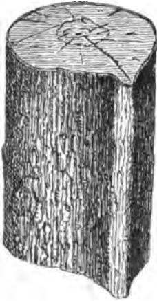
Fig. 59.—Frost-crack and frost-rib. The other cracks on the transverse section are due to desiccation.
